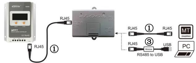
Real-time monitor the system status by the "Solar Station Monitor" software or Remote Meter.
