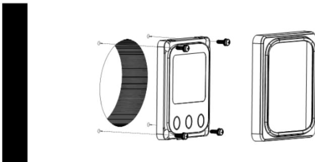
**Step1:** Locate and drill screw holes based on the installation size of the surface.
