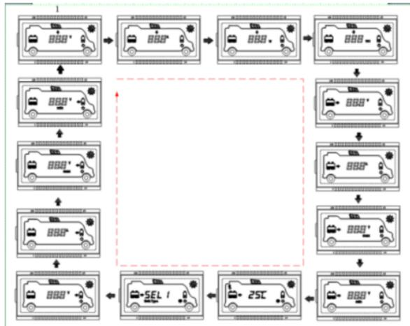
Echo Loop: PV voltage — PV current — PV power — Battery power — BATT1 voltage — BATT1 current — Max. BATT1 voltage — Min. BATT1 voltage — BATT1 temperature — BATT1 battery type — BATT2 voltage — BATT2 current — Max. BATT1 voltage — Min. BATT2 voltage — PV voltage
