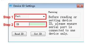
Caution: Only one of the controllers' IDs can be set at each time. Follow the same procedure to set the rest of the controllers.
