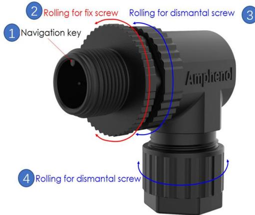
Align the plugs and sockets with the Navigation key (1) and insert the plugs. Fasten the screw (2) to secure the plug. Loosen the screw (3) to adjust the direction of the wire (every 45°), then fasten screw (3) and (4).
