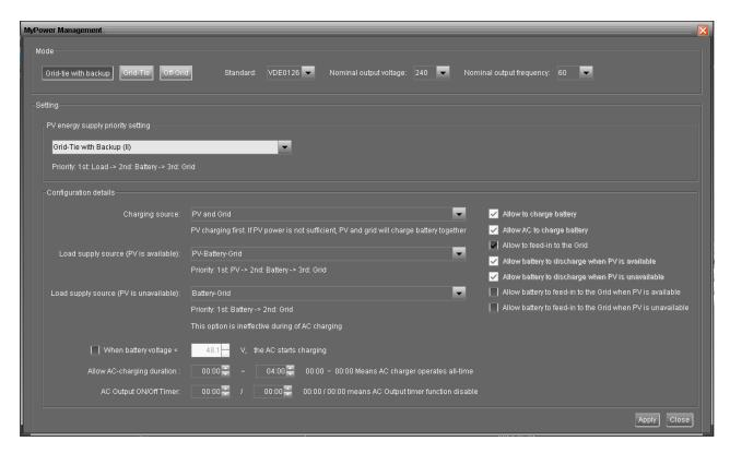
PV energy supply priority setting: 1<sup>st</sup> Load, 2<sup>nd</sup> Battery and 3<sup>rd</sup> Grid.
