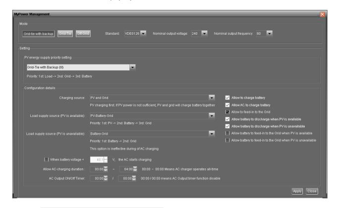
PV energy supply priority setting: 1<sup>st</sup> Load, 2<sup>nd</sup> Grid and 3<sup>rd</sup> Battery
