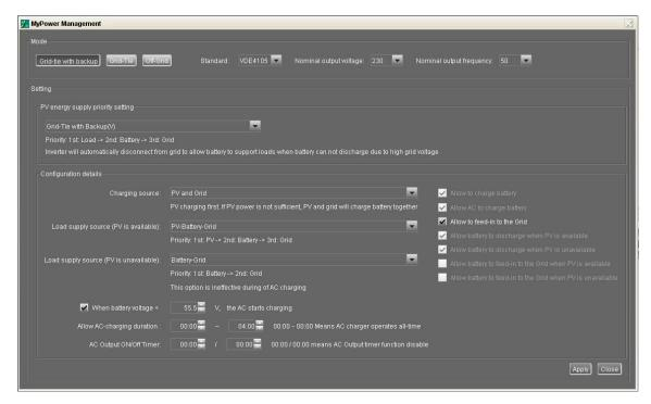
PV energy supply priority setting: 1st Load, 2nd Battery and 3rd Grid
